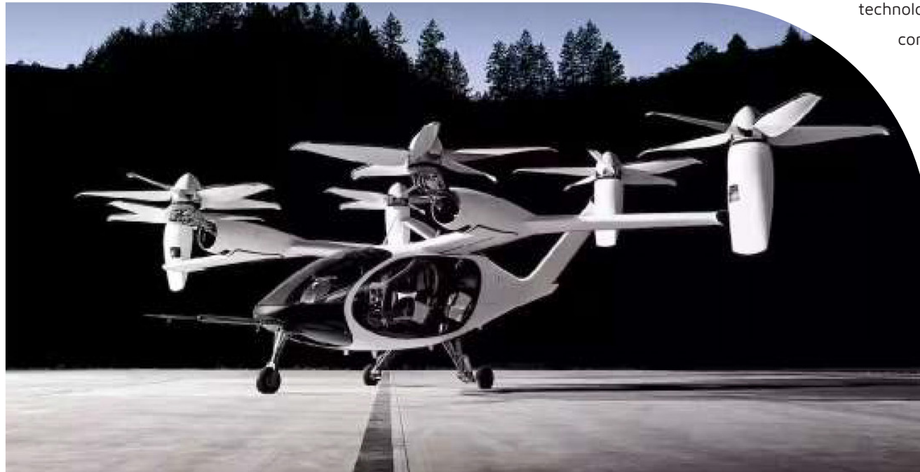
Figure 1: The Joby Aviation S-4 all-electric eVTOL, which has six electric motors to carry one pilot and four passengers, was awarded military airworthiness approval in 2020, and recently established a new certification agreement with the FAA for a more rapid commercial entry date of 2024. Image used courtesy of Joby Aviation
