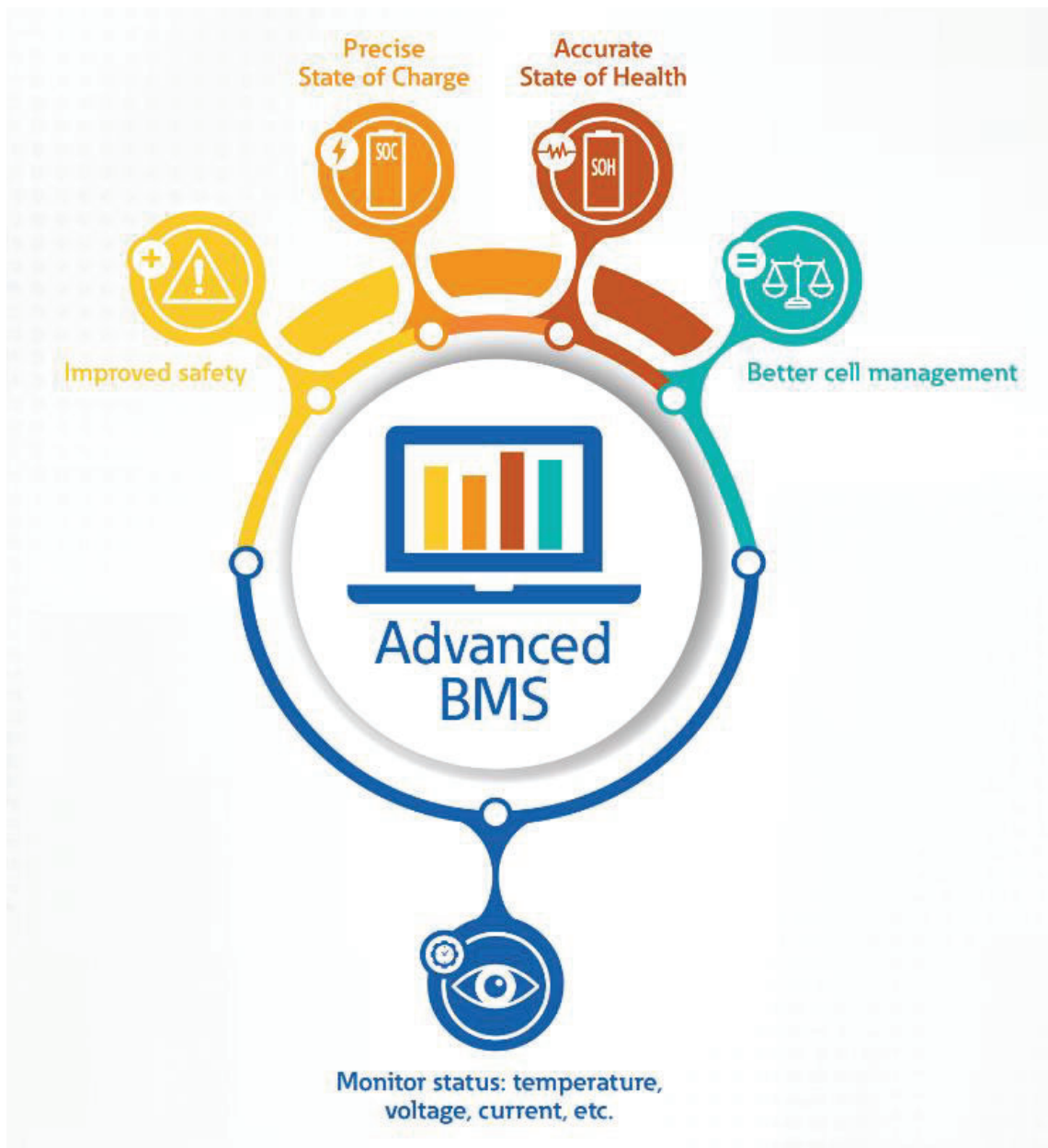
Primary functions of a BMS. (Image: Eaton.)
