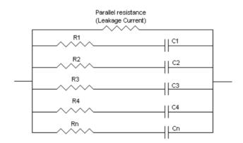
When voltage is applied current flows through each of the RC circuits. The amount of time required to charge the capacitor is dependant on the CxR values of each RC circuit. Obviously the larger the CxR the longer it will take to charge the capacitor. The amount of current needed to charge the capacitor is determined by the following equation:
