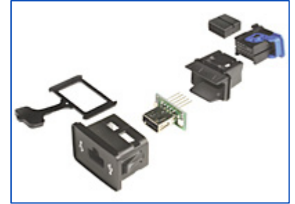
Exploded View of Present Production Illuminated USB Port
