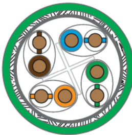
SF/UTP with cross element
